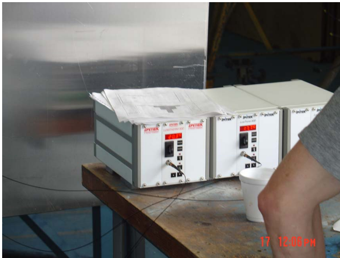
Fig. 3. Fiber optic probe cables attached to signal processing units used to monitor temperature elevations inside the microwave chamber during sample irradiation.
