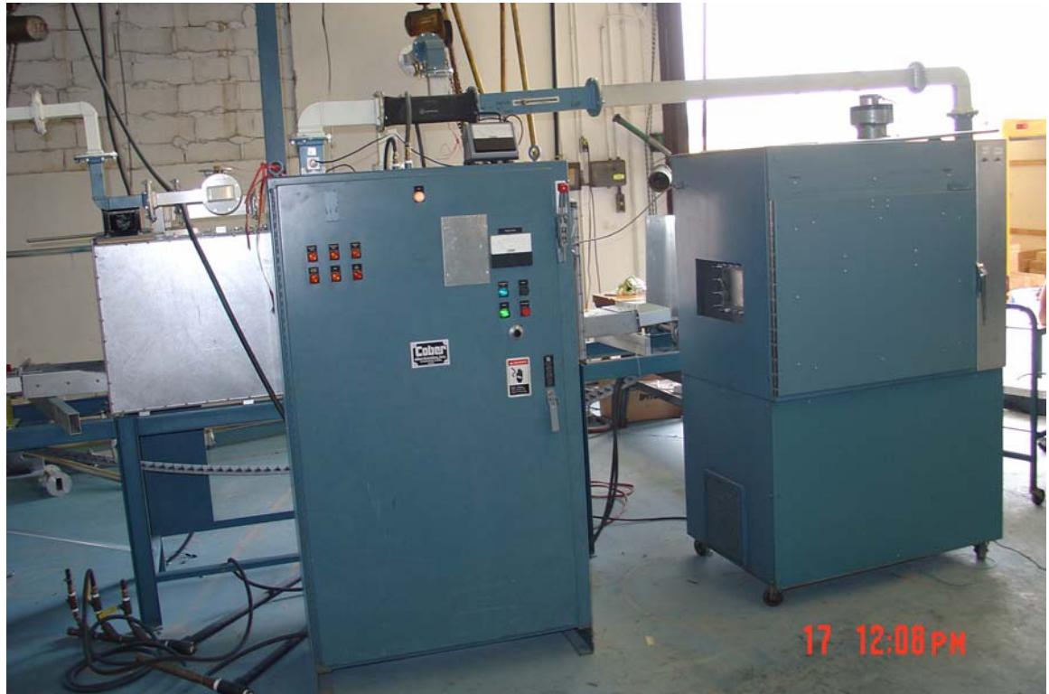
Fig. 2a – Batch microwave unit (2.45 GHz generator-left and treating chamber-right) used in experiments with 4- by 4-inch cant section samples.
