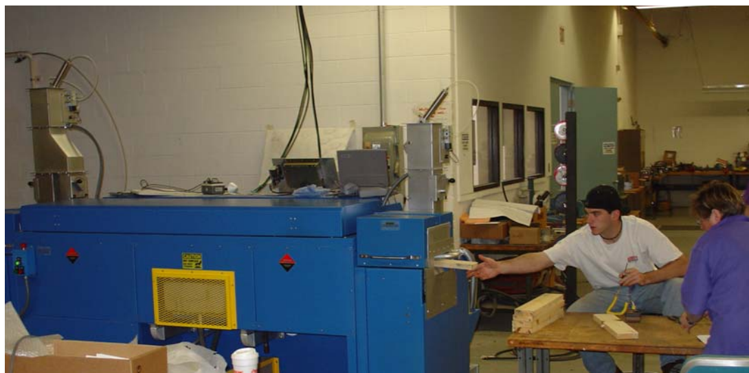
Fig. 1a – Photograph of continuous 2.45 GHz industrial microwave used for experimental trials (outfeed side with core temperature measure being taken on 1- by 4-inch board samples).
