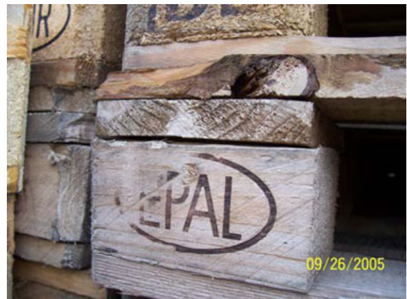
Figure 4f. "Barky" defect in pallet stringer.
