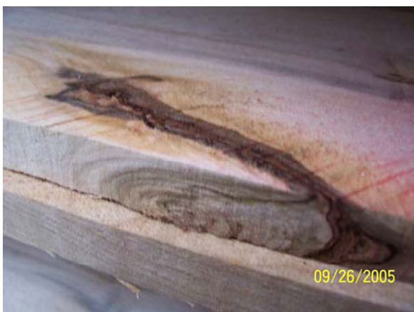
Figure 4c. Bark pocket in pallet deckboard.
