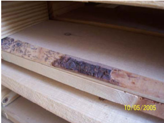
Figure 4b. Bark pocket in pallet stringer.
