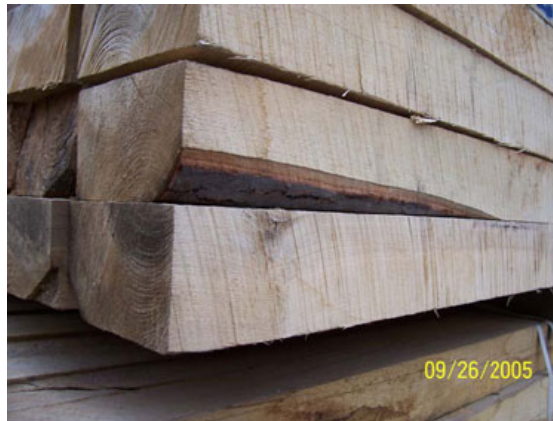
Figure 5b. Bark remnant on hardwood pallet cants in the Northeastern United States.
