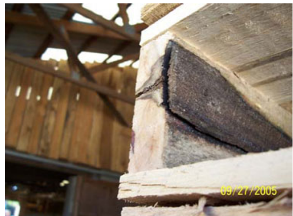
Figure 4f. "Barky" defect in pallet stringer.
