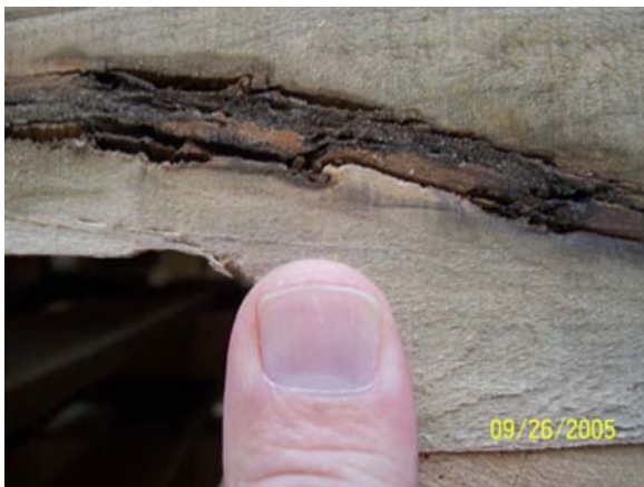
Figure 4c. Bark pocket in pallet deckboard.
