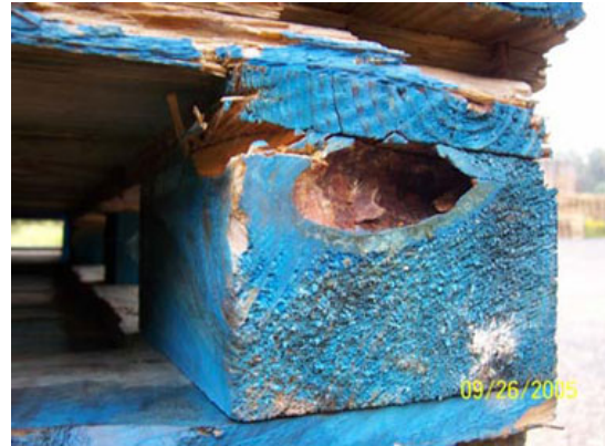
Figure 4e. "Barky" defect in pallet deckboard.
