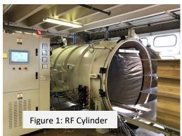
frequency can heat wood at greater depths. RF creates an electro-magnetic field that excites the water molecules present in wood, producing friction that rapidly generates internalized heat. The processes generates heat that results in the whole volume of the product being heated at once, not just the surface, which is referred to as volumetric heating. This provides an opportunity to heat large, tightly packed bundles of wood boards and cants quickly and effectively.
