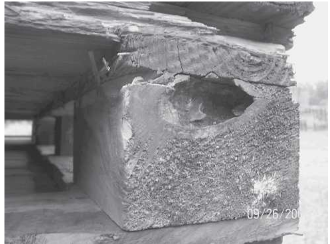
Figure 4. — Barky hole in pallet block.
