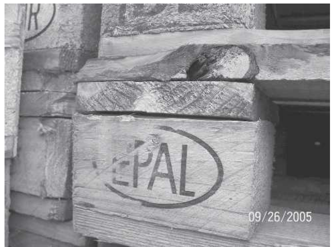
Figure 5. — Barky hole in pallet deckboard.
