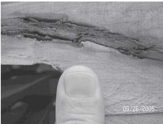
Figure 2. — Bark pocket in pallet stringer.
