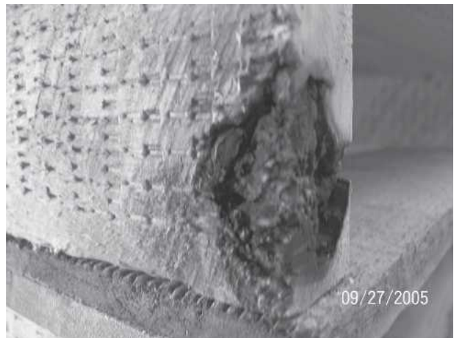
Figure 6. — Remnant loose knot on end of pallet stringer.
