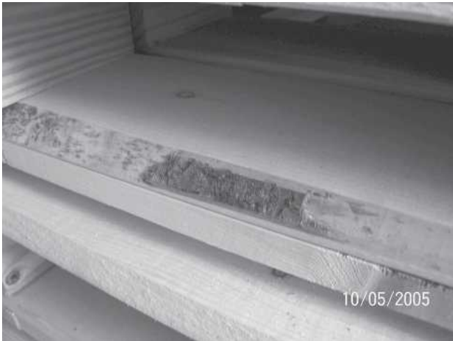
Figure 1. — Wane on board with bark occurrence not removed by debarker.
