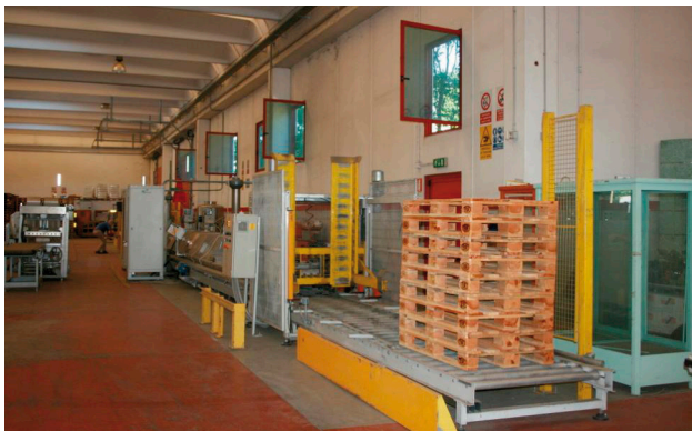
A continuous process (left) allows a constant throughput of material such as pallets. Infrared imaging can be used to monitor surface temperature and ensure temperature requirements have been met. (Photos: EMitech srl)
