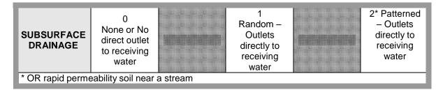
Subsurface drainage accounts for the presence of artificial drainage in a field. There are three options provided in the P Index: *None, Random,* and *Patterned*.
