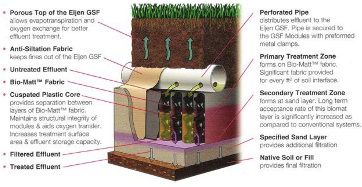
Fig. 1. Cross-section of the GSF system.
