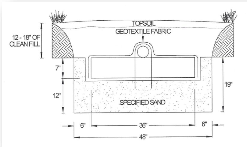
Fig. 5. Minimum dimensions for modules and sand where perc rates are between 3 and 60 min/in.
