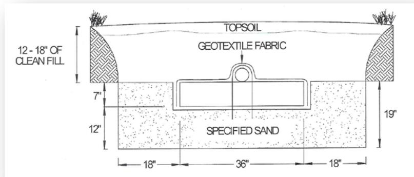
Fig. 6. Minimum dimensions for modules and sand where perc rates are between 61 and 180 min/in.
