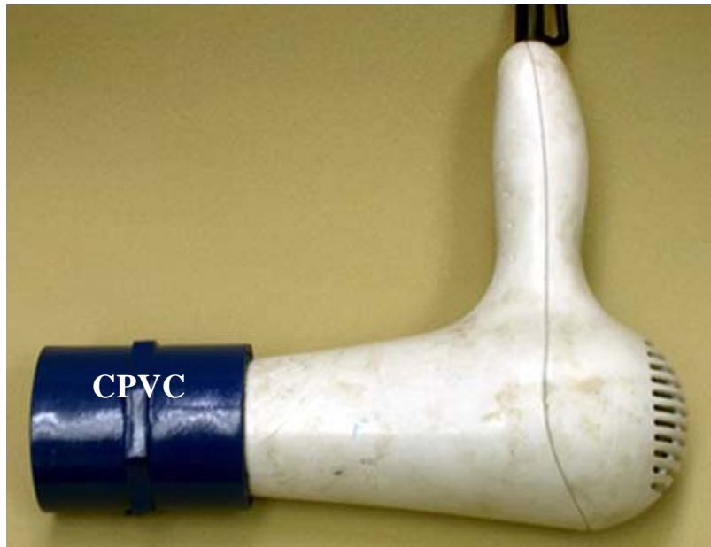
Figure 6. Blow dryer glued to the coupler which would slide onto the air entrance tube (unglued).
