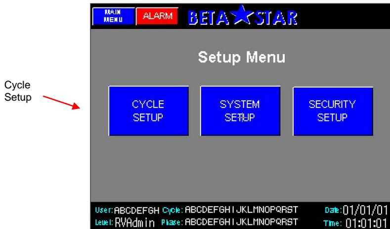
From the Setup Menu screen push the CYCLE SETUP button, this will bring up the Select Cycle to Setup screen shown below.
