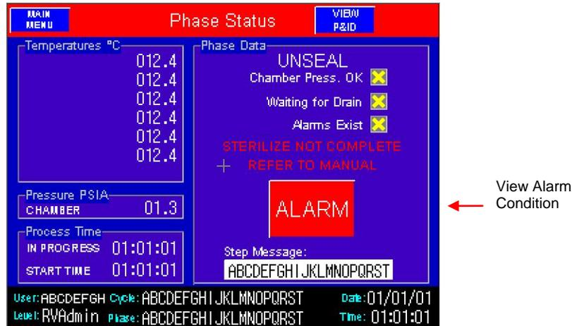
Pressing the ALARM button will bring up the Alarm Summary screen below. This screen shows all alarms that have occurred, the red alarms are active, the green alarms have been acknowledged. You can silence the audible alert by pressing the SILENCE button.
